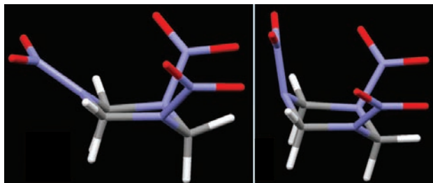
The crystal structure of RDX changes at high pressure
